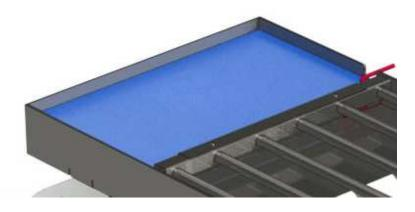
In addition, we took the care to place in it a space to vibrate from 1 to 3 moulds, depending on its sizes. Its polyurethane sanitary cloth is easy to clean and does not dry out in contact with chocolate.
